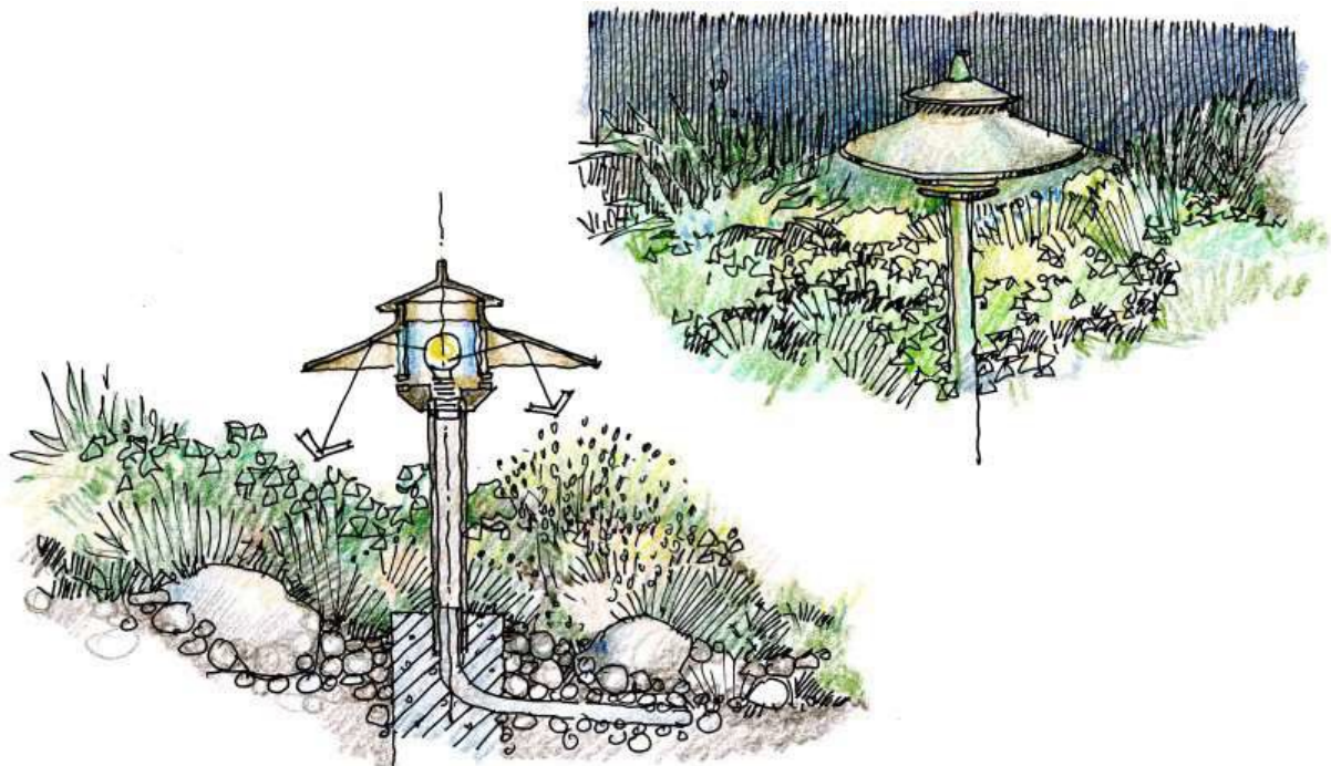
Fixture designs are downward facing with horizontal cut-offs to minimize light spill
